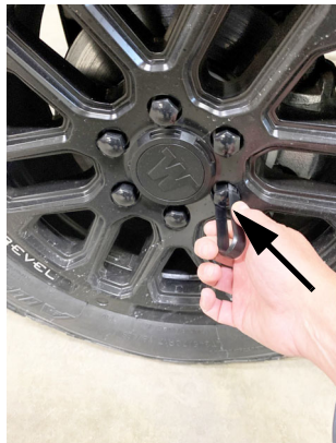
Use the tool to remove the protective caps prior to removing the lug nuts. -Typical View
